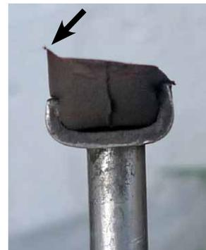
Fig. 2: If a ridge (arrow) appears on your brake pad, then it is not hitting the rim squarely. Adjust the brake pad immediately to prevent the tire from being cut.
