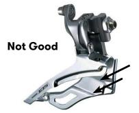
Front derailleurs for doubles have smooth inner cages that work well with all chainring combinations. Also recommended for triple cranks. Front derailleurs for triples have steps in the cage (arrows) that must line up with the chainrings. With custom chainring combinations, they may not work well.
