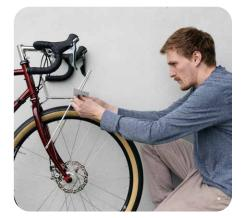
Check your alignment before you tighten the stays. Double-check it after the bolts are tight. On the UD-1, you don't want to cut the stays to the wrong length!
