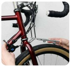
Install the rack platform. If the fork crown is too deep, you can use a recessed brake nut in many cases (see last page).
