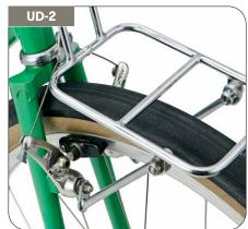
The UD-2 stays attach to the brake pivots with Rene Herse rack bolts (included). The stays come in two lengths (150 and 170 mm) to fit a wide range of bikes.
