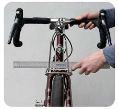
Level the rack from side to side as well. A ruler helps, because it exaggerates the angle of the rack.
