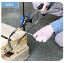
Remove the stays and cut them to the correct length with a hacksaw. The stay needs to be held firmly for a clean cut.
