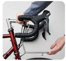
Pull or push the rack until the platform is level. For bikes with fenders, you may prioritize a good fenderline over a level rack (see last page).
