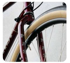
Requirements: All racks: Fork crown with a hole all the way through. UD-1: eyelets somewhere on the fork. UD-2: cantilever brakes that end flush with the posts.
