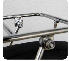
The rack stays should protrude slightly from the eyebolts, but not extend above the rack platform.
