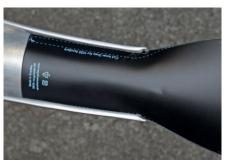
Insert the other edge of the mudflap into the rolled fender edge. Flatten the mudflap. If the mudflap cannot be flattened, it's too wide. Remove and trim.
