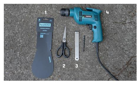
1 Rene Herse Mudflap 2 Scissors 3 Rene Herse Fender Edge Tool 4 Drill with 5 mm bit
