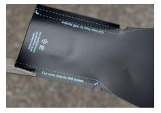
For narrower fenders, cut the mudflap to fit. (Lines marked 'H-40' are for H-50 fenders. 'H-30' lines are for H-40 fenders. Sorry about the typos.) Replicate the cutouts for the fender corners.
