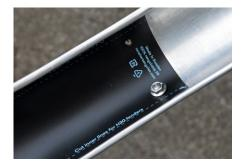
Install the fender eyebolts as you normally would. Pro Tip: If the mudflap doesn't reach the fender bolts, you can still use the mudflap. The cutouts at the fender corners will hold it in place.
