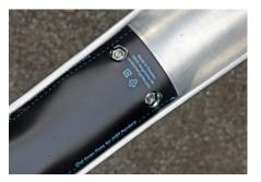
Now the mudflap fits over the 8 mm nuts for the fender eyebolts. To remove the mudflap, push up the center, starting at the fender end. Carefully pull the mudflap out of the fender edges.
